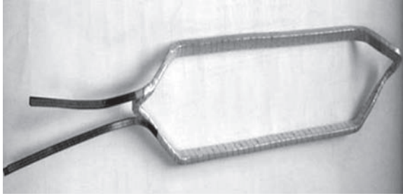
Figure 4.4 Wound-formed multi-turn coil
