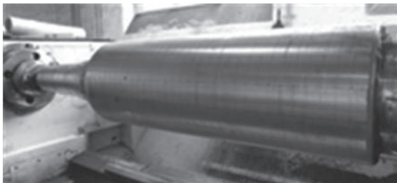
Figure 4.1 Example of a SPM rotor for a high-speed motor. © 2017 IEEE. Reprinted, with permission, from [4]
